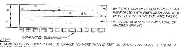
1) CONSTRUCTION JOINTS SHALL BE SPACED NO MORE THAN IZ FEET ON CENTER AND SHALL BE EQUALLY SPACED OVER THE LENGTH AND WIDTH OF THE PAD. CONSTRUCTION JOINTS SHALL BE CUT OR FORMED IN ACCORDANCE WITH AMERICAN CONCRETE INSTITUTE STANDARDS AND JOINT SEALANT RECOMMENDATIONS.
