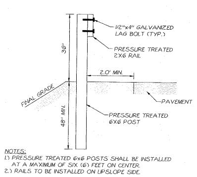
Typical Wood Guide Rail Detail
