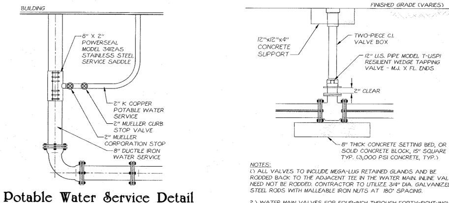
L) ALL VALVES TO INCLUDE MEGA-LUG RETAINED GLANDS AND BE RODDED BACK TO THE ADJACENT TEE IN THE WATER MAIN. INLINE VALVES NEED NOT BE RODDED. CONTRACTOR TO UTILIZE 3/4" DIA. GALVANIZED STEEL RODS WITH MALLEABLE IRON NUTS AT 180° SPACING.
