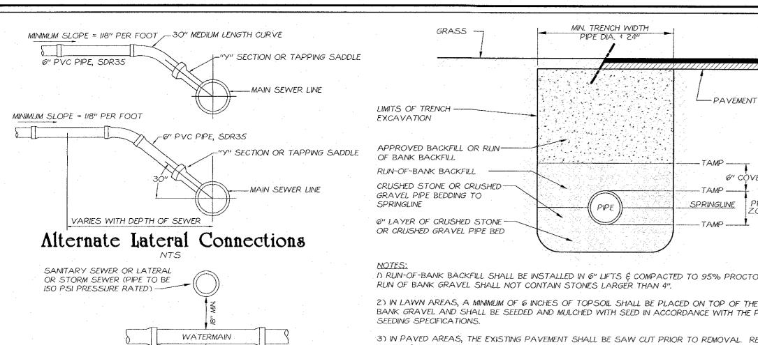
. I) RUN-OF-BANK BACKFILL SHALL BE INSTALLED IN 6" LIFTS & COMPACTED TO 95% PROCTOR DENSITY.
