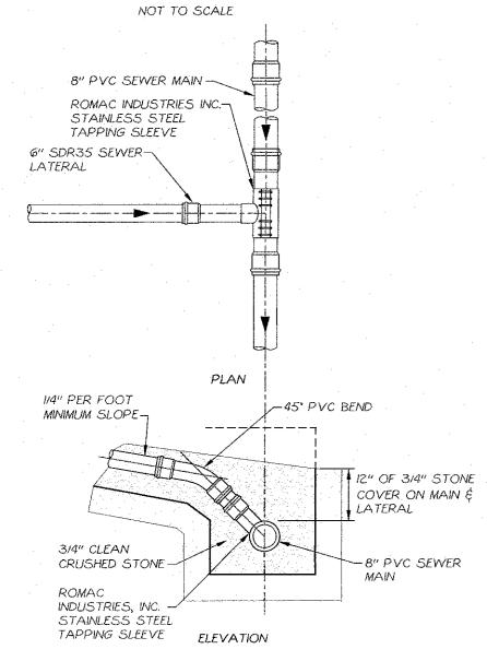
1.) FIELD LOCATION AND ALIGNMENT OF NEW SADDLE TO BE APPROVED BY THE TOWN OF NEWBURGH WATERISEWER SUPERINTENDENT PRIOR TO INSTALLATION. 2.) NEW STAINLESS STEEL TAPPING SLEEVE ON EXISTING SANITARY SEWER MAIN IN ACCORDANCE WITH MANUFACTURER'S REQUIREMENTS, TOWN OF NEWBURGH CODE,
