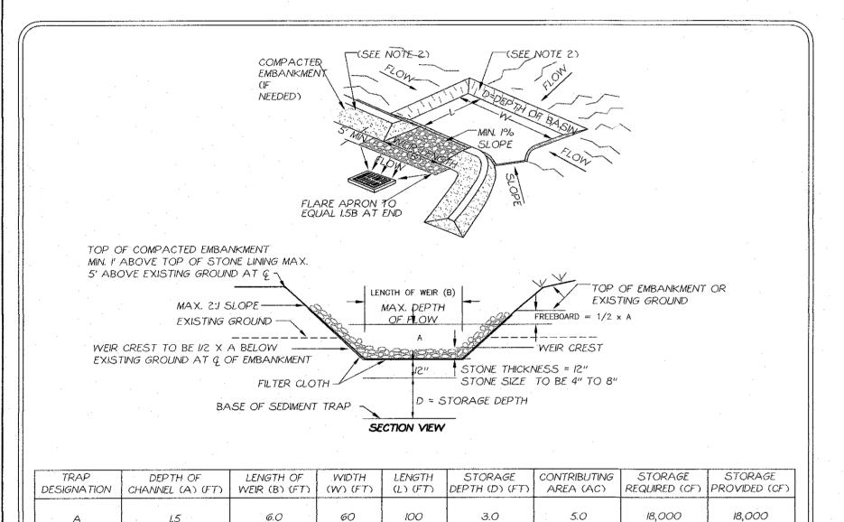
I) THE AREA UNDER THE EMBANKMENT SHALL BE CLEARED, GRUBBED, AND STRIPPED OF ANY VEGETATION AND ROOT MAT. TOP OF EMBANKMENT SHALL BE A MINIMUM OF FOUR (4) FEET WIDE.
