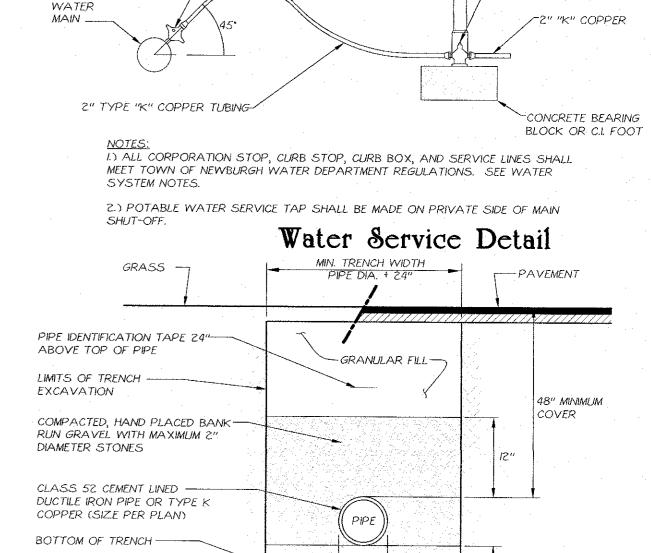
I) GRANULAR FILL SHALL CONSIST OF SELECT GRANULAR FILL OR SUITABLE ON-SITE EXCAVATED SOIL (LARGEST STONE SHALL BE LESS THAN 3"). GRANULAR FILL SHALL BE INSTALLED IN 6" LIFTS & COMPACTED TO 95% PROCTOR DENSITY.
