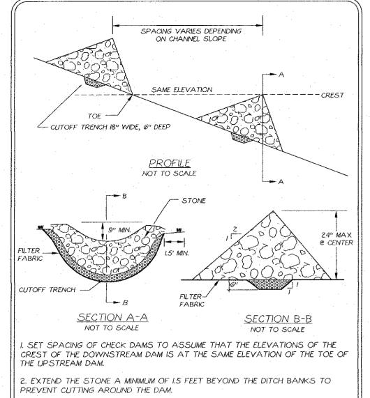
3. INSTALL IN ROAD SWALES AFTER SWALE IS SHAPED. CHECK DAMS SHALL BE MAINTAINED UNTIL ROAD IS PAVED & SWALES ARE STABILIZED. REMOVE
