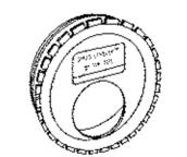
1. INSERT A SPEED LEVELER IN THE END OF ALL OUTLET PIPES IN THE DROPBOX. 2. ROTATE UNTIL EFFLUENT ENTERS ALL OUTLETS EQUALLY. WOODARD'S SPEED LEVELER FSL-4
